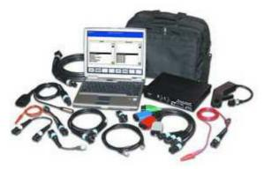
The OmiPro series is an integrated PC-based diagnostic solution for Rover and Land Rover vehicles. OmiPro is supplied with factory-installed software and technical data, covering a wide range of vehicle models. It provides the opportunity to diagnose faults reported by vehicle control modules and view 'live data' parameters in real time. The OmiPro allows the professional technician to read and clear faults on engine management, airbag, ABS and other
