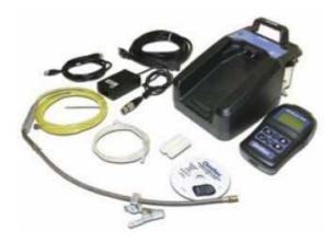
5 gases Measured HC, CO, CO2, NOx, O2 Measurement accuracy meets or exceeds requirements for OIML Class 0 and BAR97 Lambda and Air Fuel Ratio measurement. Very Fast Warm up and Response Times. Battery powered – Up to 4 hours continuous use, charge time 4 hours max. Battery Charger included. Wireless Bluetooth Handset with range in excess of 30 feet.
