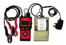
within the plates and plate separators. Conductivity is measured by probing the battery with a small AC current ripple that generates a small AC voltage response. And is the relative ratio of the variation in current with the variation in voltage. By using this method to test and analyze the conditions of the 12V battery means the battery can be tested and analyzed whether it is on or off the vehicle. This means you don't need to disconnect the battery from the vehicle.
